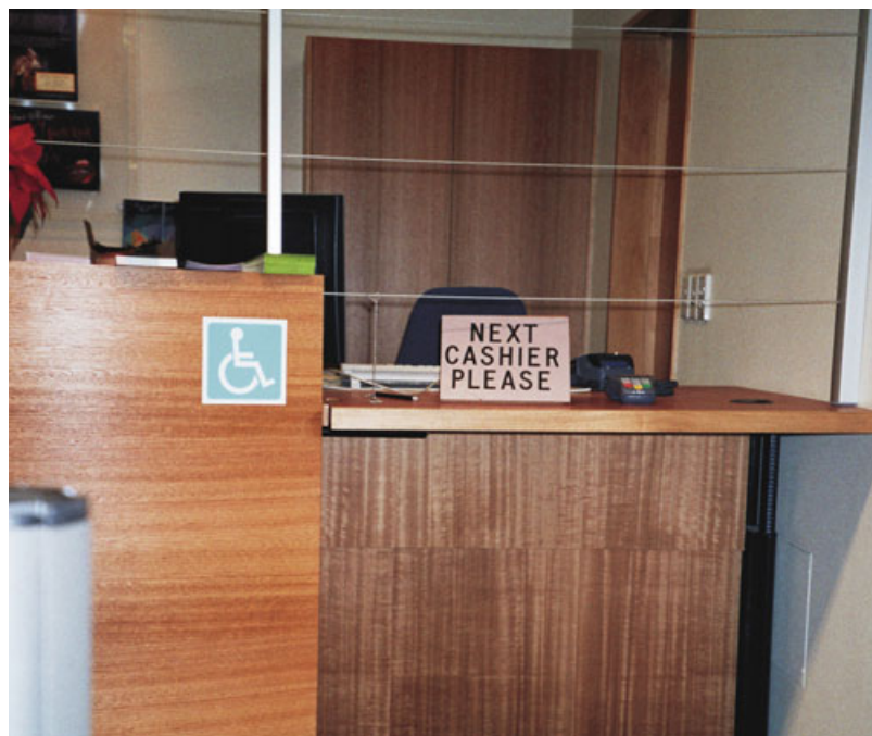
An accessible counter that is not used because the cashier operates from another part of the counter.
