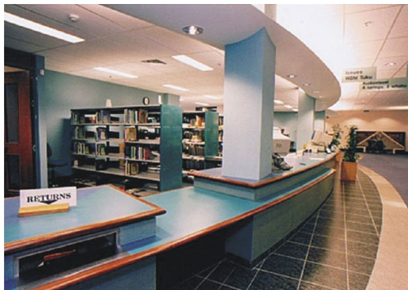
A good design but the pillar affects usability. The action is in the centre of the counter.
