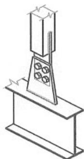
**Figure 1.** Example of unstiffened eccentric cleat connection
