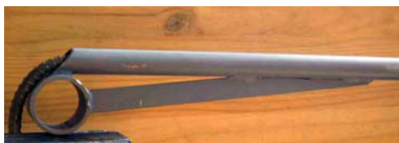
Figure 1: A 12 mm bar bent to correct diameter of 60 mm. Source: CCANZ IB79.
