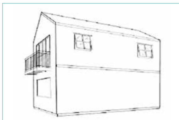
Home showing typical cantilevered balcony
