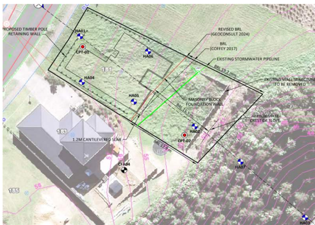
Figure 2. Site plan showing ground contours, BRL, revised BRL and location of dwelling (Source: Owner's geotechnical report)
