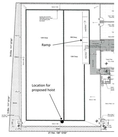
Figure 1: Plan showing ramp as approved, and the location of the proposed hoist (not to scale).
