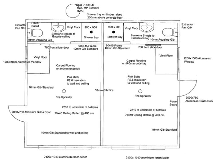
Figure 2: Floor plan of the converted garages (Not to scale)
