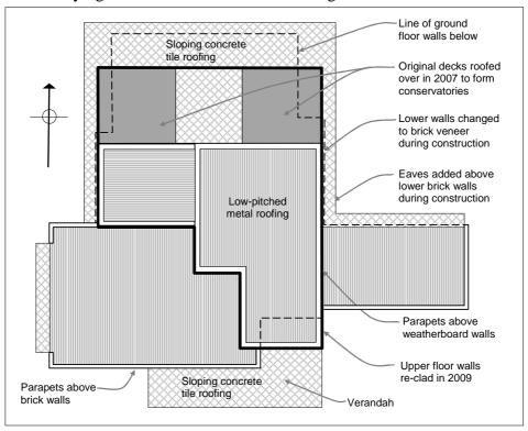
2.3 Except for a small gable to the north, the upper level roof is low-pitched profiled metal, with the upper walls forming parapets. Lower level roofs are a mix of low-pitched profiled metal with some parapets and 25° pitched concrete tile lean-to roofs.
