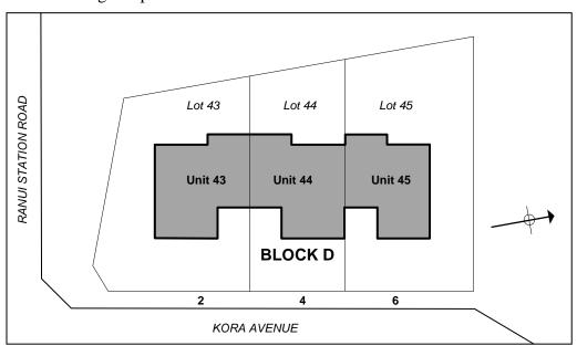
3.2 Block D is a two storey building, which is situated on a gently sloping site in a low wind zone in terms of NZS 3604<sup>2</sup>. The block sits at the corner of Kora Avenue, with the main entries and garage doors facing east towards the road. The building is fairly
