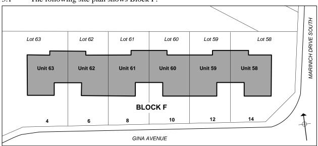
3.2 Block F is a two-storey building situated on a gently sloping site in a low wind zone in terms of NZS 3604<sup>3</sup>. The block sits at the corner of Gina Avenue, with the main entries and garage doors facing south towards the road. The building is fairly simple in plan and form, with garages set back from the front wall. The ground floor
