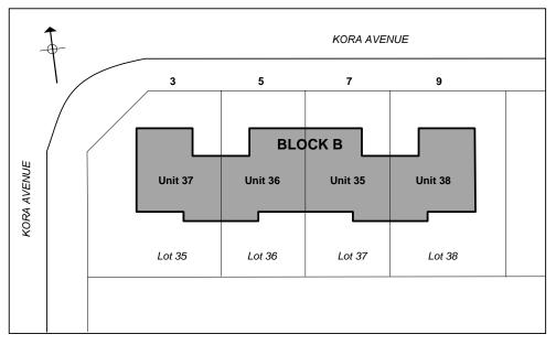
3.2 Block B is a 2-storey building, which is situated on a flat site in a low wind zone in terms of NZS 3604<sup>3</sup>. The block sits on the corner of Kora Avenue, with the main entries and garage doors facing north towards the road. The building is fairly simple in plan and form, with garages set back from the front wall. The ground floor
