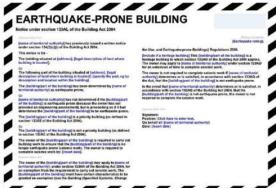
(left) EPB notice, black and white border. Earthquake rating 20% to less than 34%. The risk of failure under seismic load is approximately 10-25 times the risk of failure for buildings that are 100%NBS.
