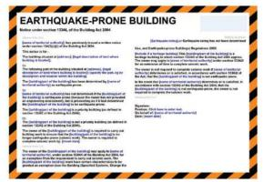
(left) EPB notice, orange and black border. Earthquake rating 0% to less than 20% or where no engineering assessment is provided. If the building has an earthquake rating of less than 20% the risk of failure under seismic load is approximately more than 25 times the risk of failure for buildings that are 100%NBS.
