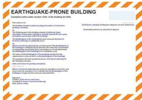
(left) **Exemption notice.** Buildings or parts assessed as earthquake prone but owners exempted from carrying out seismic work. Exemption notices must be attached in a prominent place on or adjacent to the building.
