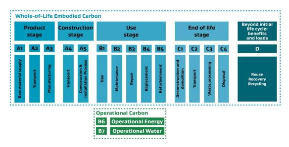
Emissions in all modules fall within the scope of this methodology, with the exception of modules *B6 Operational energy* and *B7 Operational water*, as shown above.
