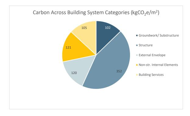
The following chart shows embodied carbon per m<sup>2</sup> GFA Total (kgCO<sub>2</sub>e/m<sup>2</sup>) across the life cycle stages.
