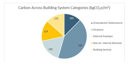
The following chart shows embodied carbon (Gross) per m<sup>2</sup> GFA Total (kgCO<sub>2</sub>e/m<sup>2</sup>) across the life cycle stages.
