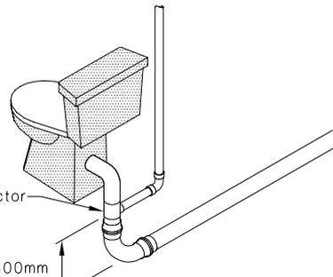
**2) Discharge pipes serving soil fixtures connected individually to the drain or to a stack and utilising a fixture vent**
