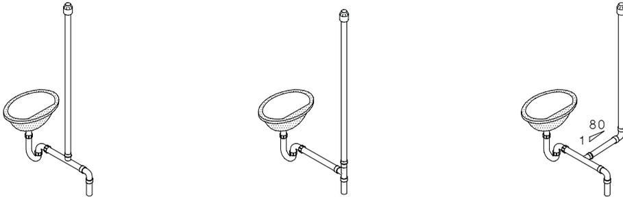
**(a) Vertical and/or graded fixture vent pipe open at its upper end**
