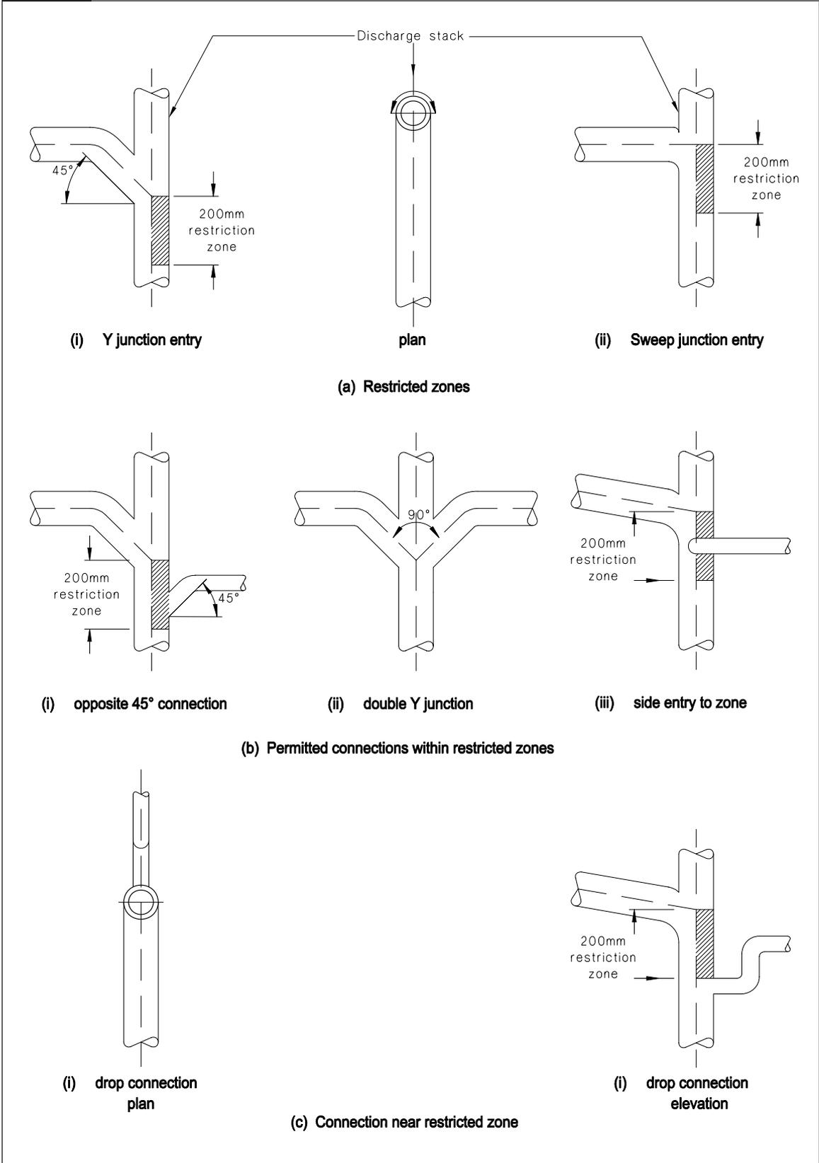
**Figure 10: Acceptable methods of vent pipe installation**
