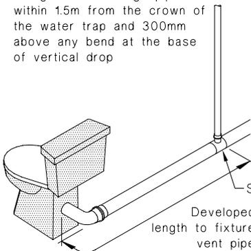
d) S or P trap non vented pan, fixture vent connected to the vertical discharge pipe as for c)
