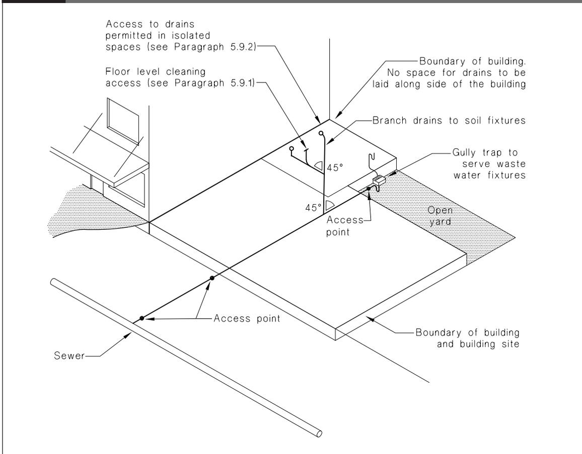
**5.9.3** *Access points* may be located in a space containing a *soil fixture*.
