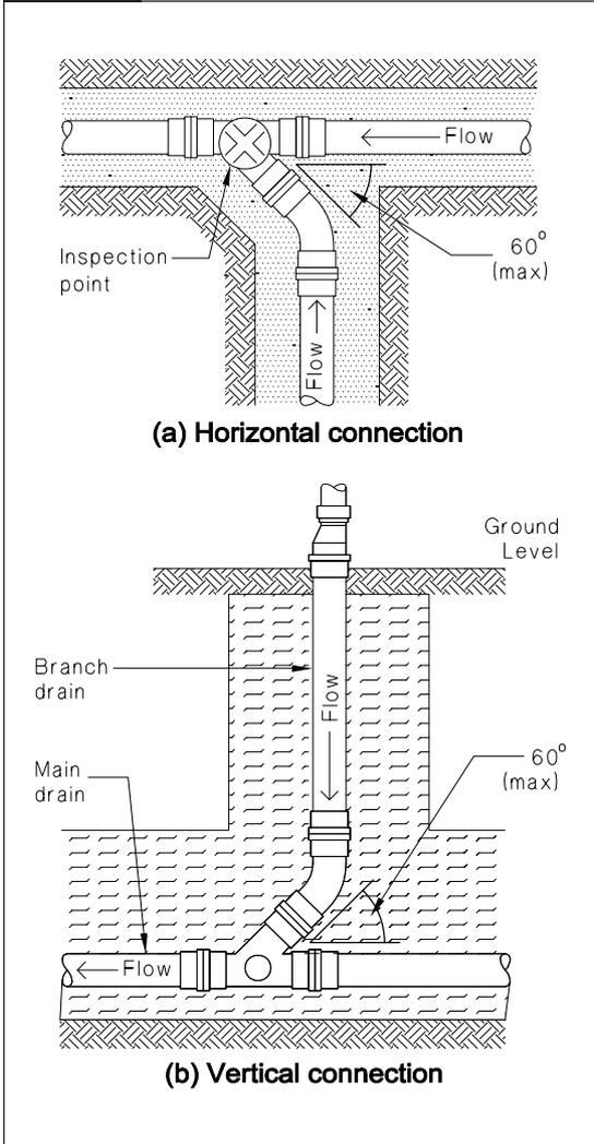
**Figure 2: Details of gully traps**
