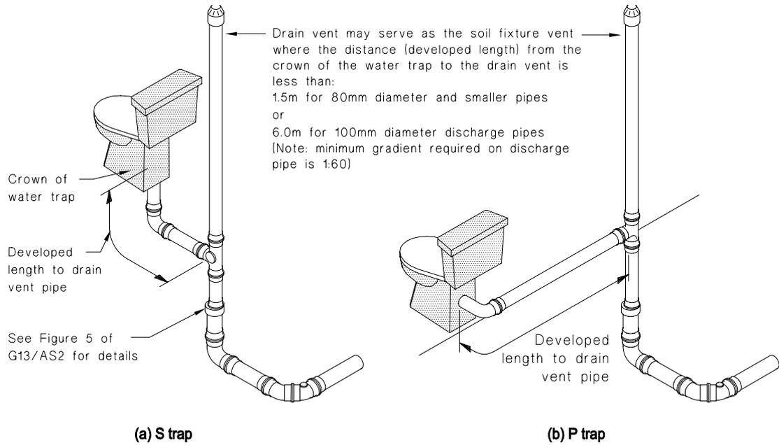
**1) Discharge pipes serving soil fixtures connected individually to the drain and utilising a drain vent as fixture vent**
