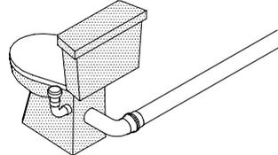
c) S or P trap non vented pan, fixture vent pipe connected to the graded discharge pipe within 1.5m from the crown of the water trap and 300mm above any bend at the base of vertical drop
