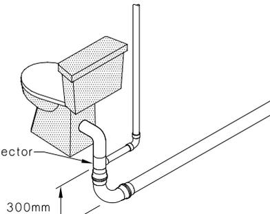
**2) Discharge pipes serving soil fixtures connected individually to the drain or to a stack and utilising a fixture vent**
