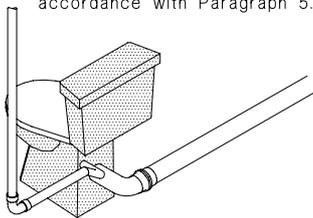
b) S or P trap pan, air admittance valve fitted to pan horn, valve to be installed in accordance with Paragraph 5.8 (valve must be vertical and secured in place)
