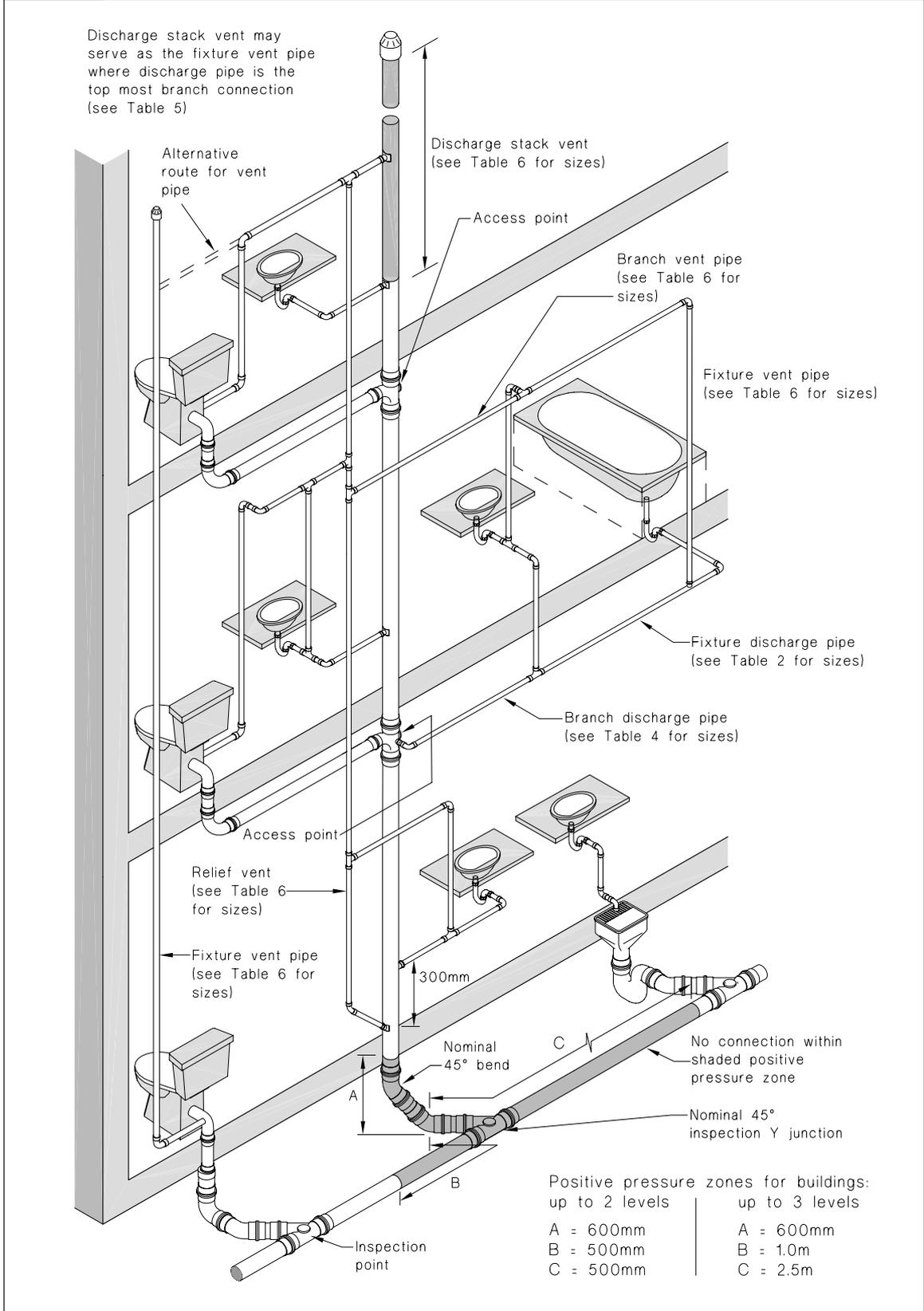
**Figure 8: Graded discharge stack**
