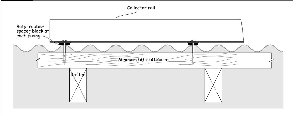
**Figure 11:** Direct fixed strap with rail – elevation
