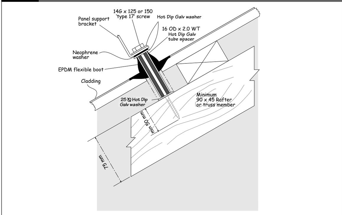
**Figure 15:** Bolt fixing
