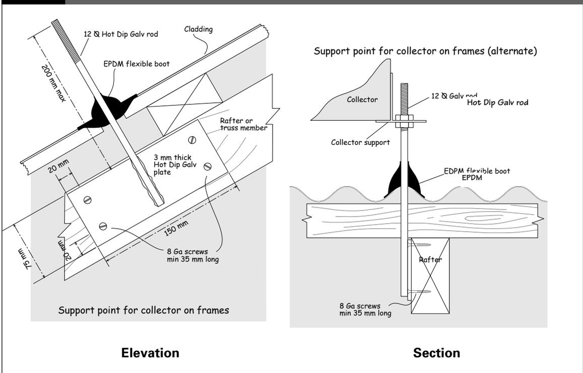
**Figure 17:** Collector support rails across roof slope
