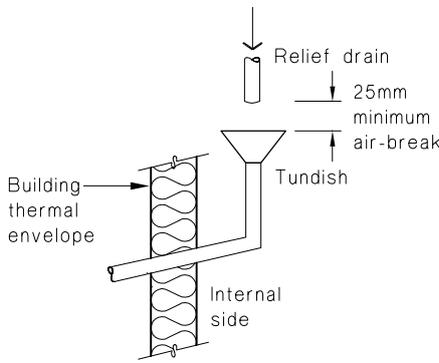
**(b) Relief drain located where freezing likely**
