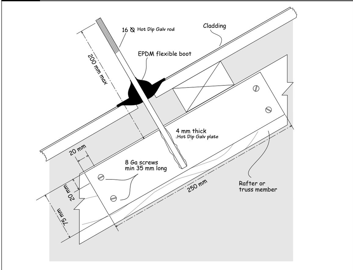
**6.6.3** The edge of the panel elevated above the roof plane is to be supported by hot dip galvanized steel or stainless steel angle struts which are:
