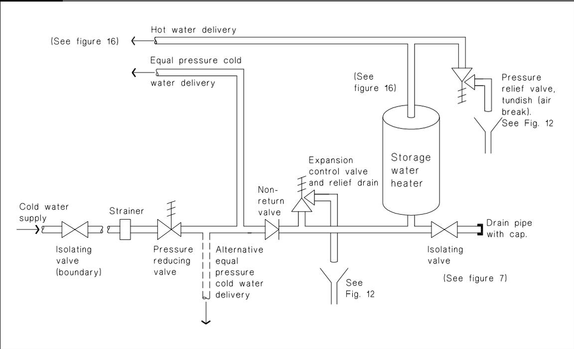
**Figure 11: Free Outlet System (push through)**
