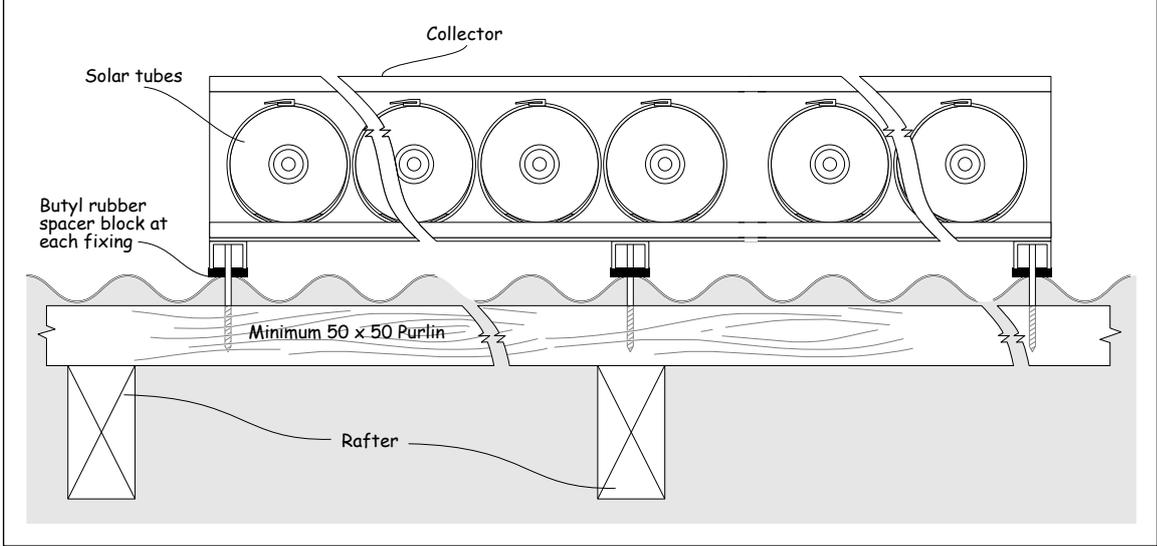
**Figure 13: Direct fixed channel – elevation**
