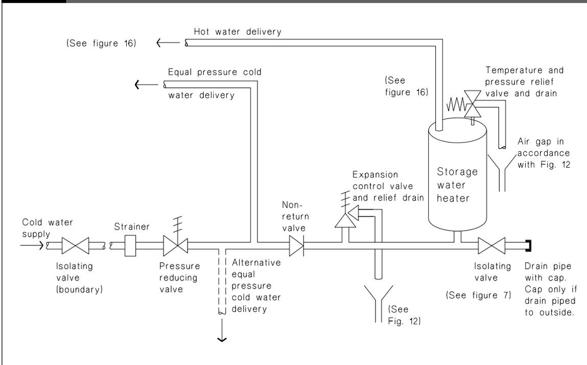
**Figure 10: Low Pressure Valve – Vented Storage Water Heater System – Pressure Relief Valve**
