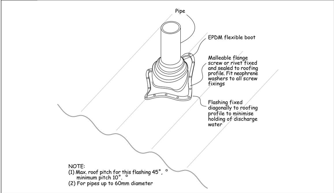
**Figure 7: Soaker flashings for penetrations (profiled metal roofs)**
