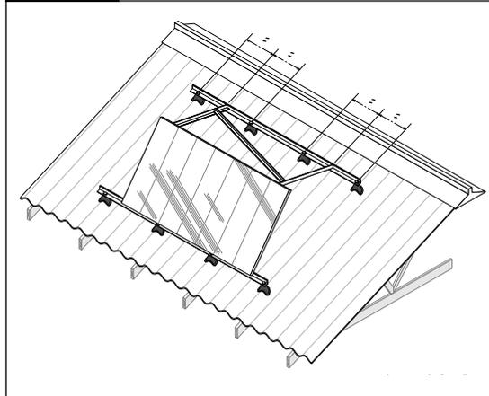
**Figure 20:** Stud fixing for panels at different pitch
