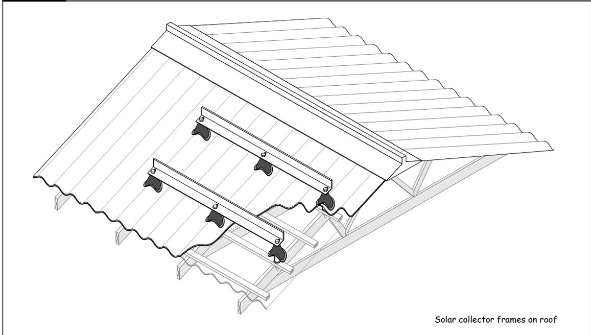
**Figure 18:** Collector frame up slope of roof
