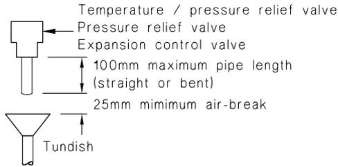
**(a) Storage water heater located where freezing likely**
