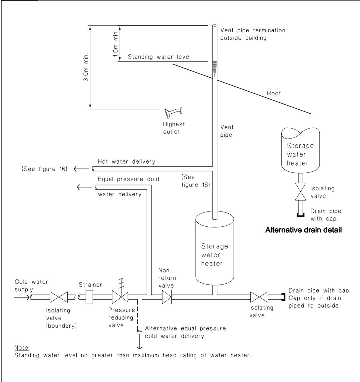
**Figure 8: Mains Pressure Storage Water Heater System (unvented)**
