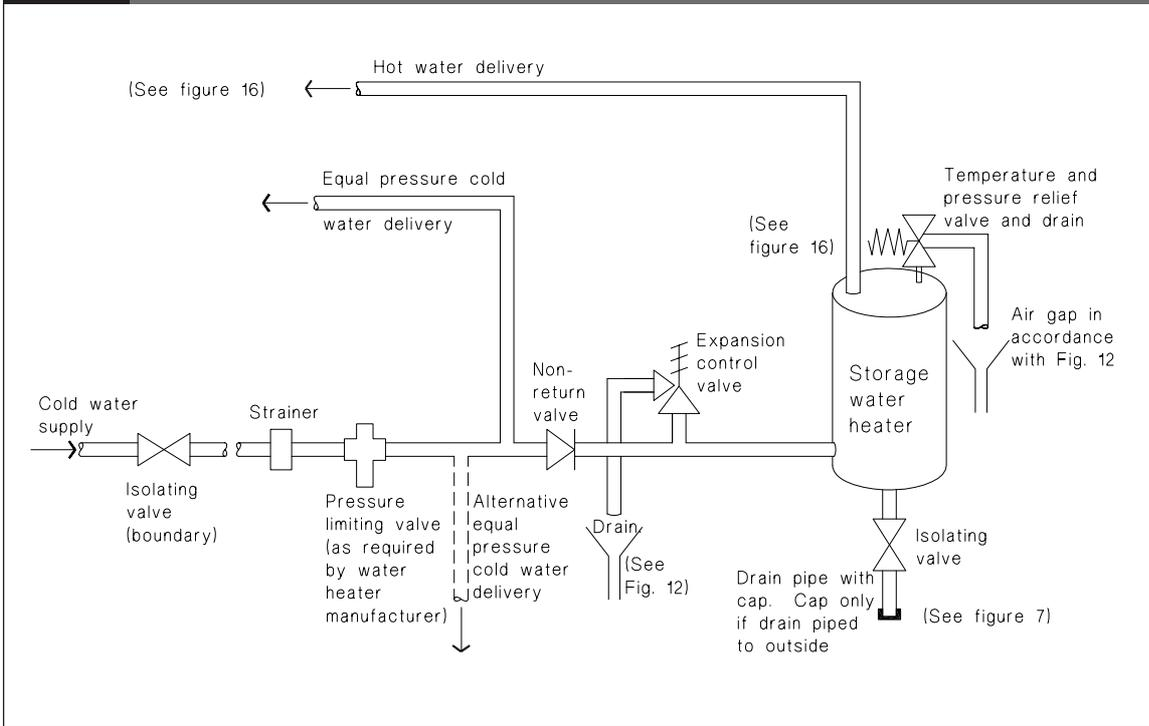
**Figure 9: Low Pressure Valve – Vented Water Heater System – Temperature and Pressure Relief Valve**
