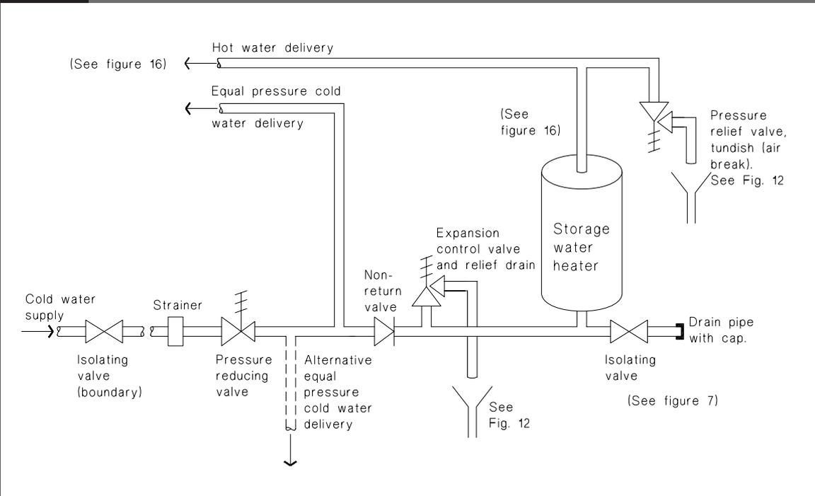
**Figure 11: Free Outlet System (push through)**
