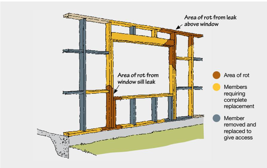
Figure 2. Damage caused by leaks from above and from window sill requiring 100% replacement of window sill
