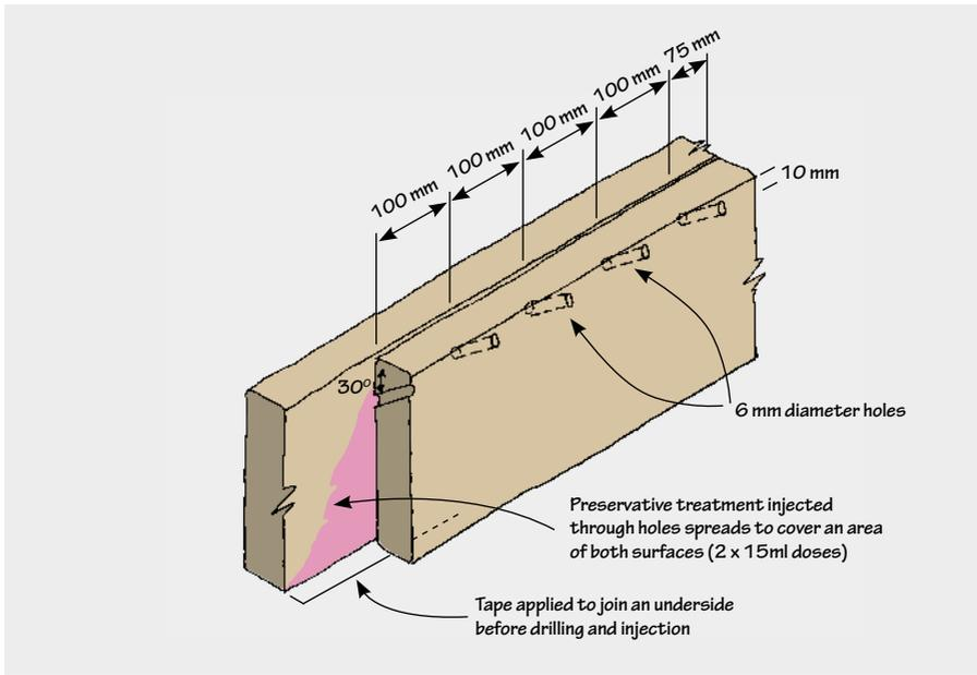
**Figure 8. Application of treatment to attached lintels**
