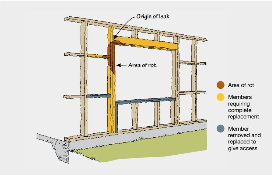
Figure 1. Damage caused by leak at end of head flashing
