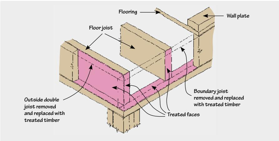
Figure 5. Boundary joist and outer joist removed to apply treatment
