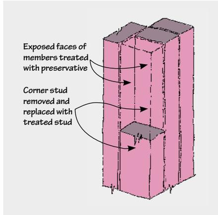
Figure 4. Corner stud removed to apply treatment
