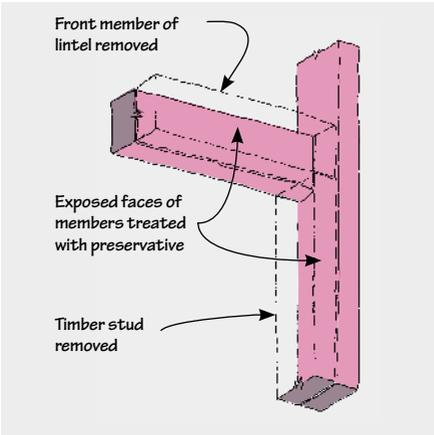
**Figure 3. Lintel and trimmer removed to apply preservative treatment**
