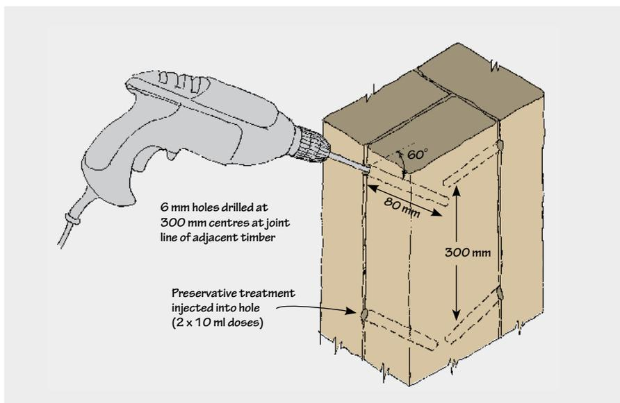
**Figure 7. Drill holes for application of treatment between timber surfaces**
