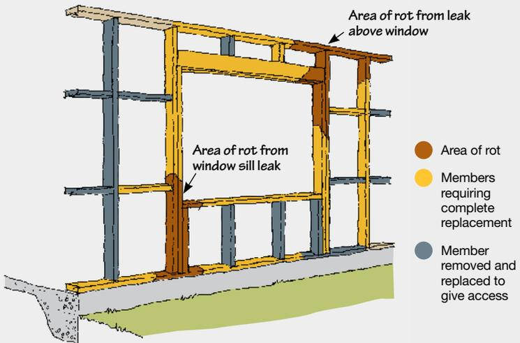
Figure 2. Damage caused by leaks from above and from window sill requiring 100% replacement of window sill
