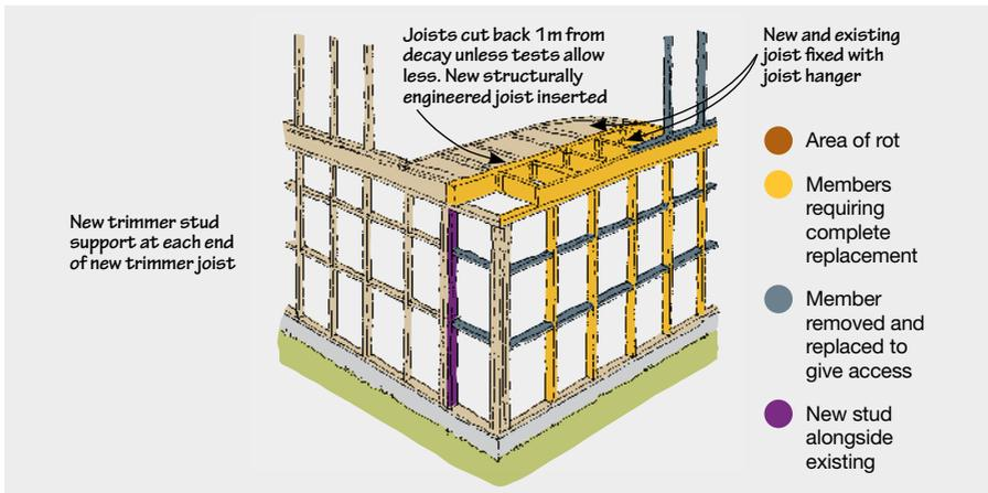
Figure 6b. New trimmer joists and joist ends inserted
