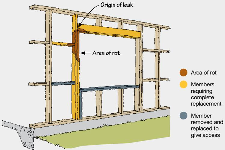
Figure 1. Damage caused by leak at end of head flashing
