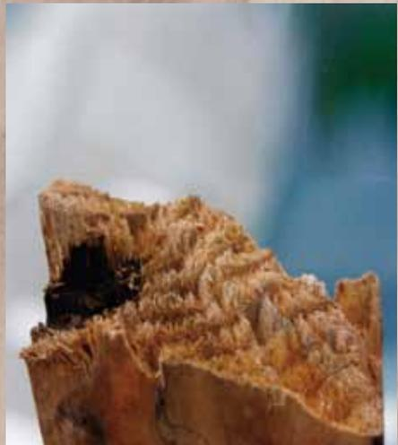
5. Fracture surface of timber with soft rot
