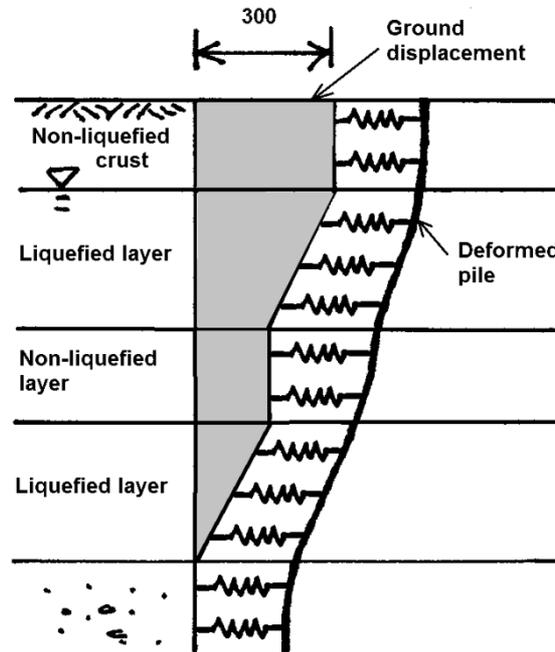
Figure 2. Example of free-field ground displacement for two liquefied layers separated by a non-liquefied layer.
