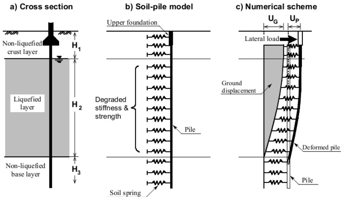
Figure 1. Pseudo-static analysis procedure for piles with lateral spreading.
