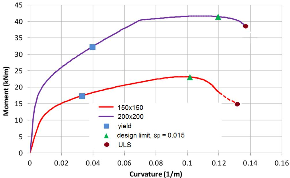
Figure 3. Example moment-curvature<sup>3</sup> relationship for small pre-stressed concrete piles (with 100 kN axial load).
