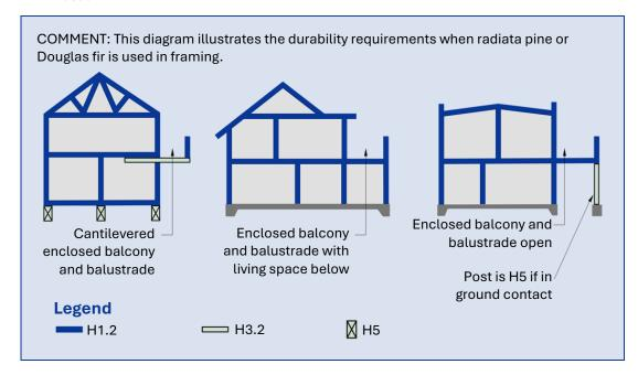
Table 1C: Requirements for radiata pine and Douglas fir solid timber to achieve a (minimum) 50 year durability performance: C – Members protected from the weather but exposed to ground atmosphere (see section 108 of NZS 3602)
