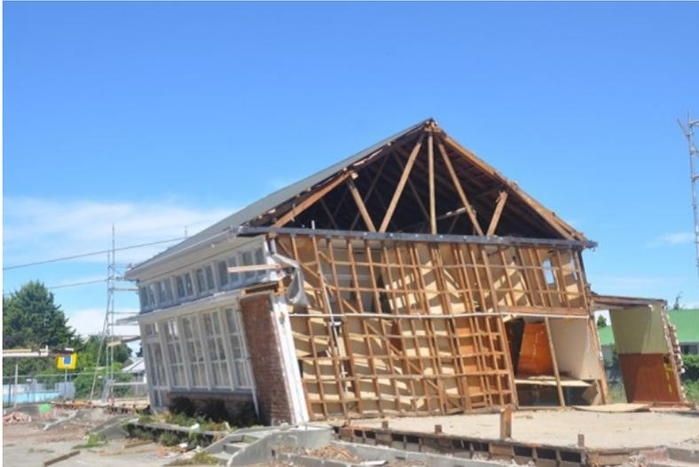
**Figure C9A.1: Transverse test of the Dominion block showing high levels of drift**
