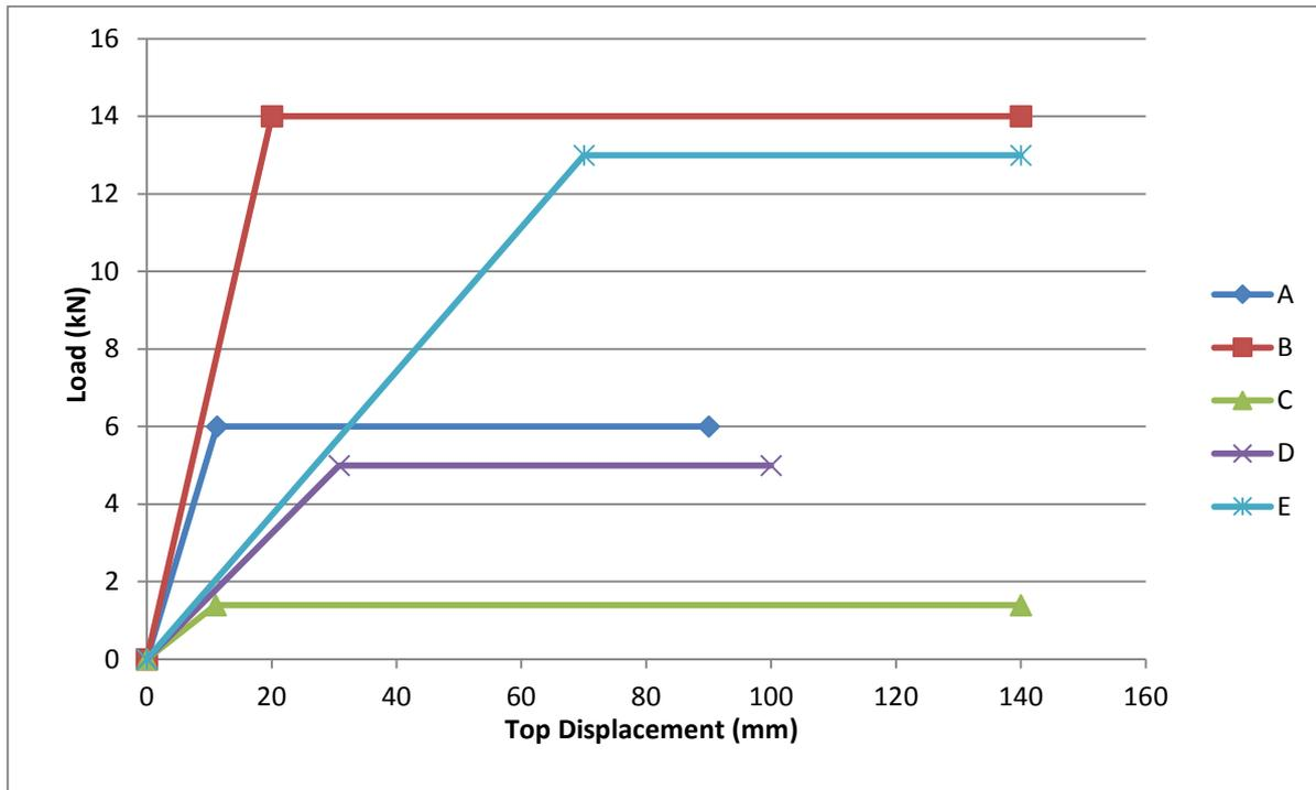
**Figure C9B.1: Capacity relationships for timber framed walls with typical sheathing materials, for heights as noted below**
