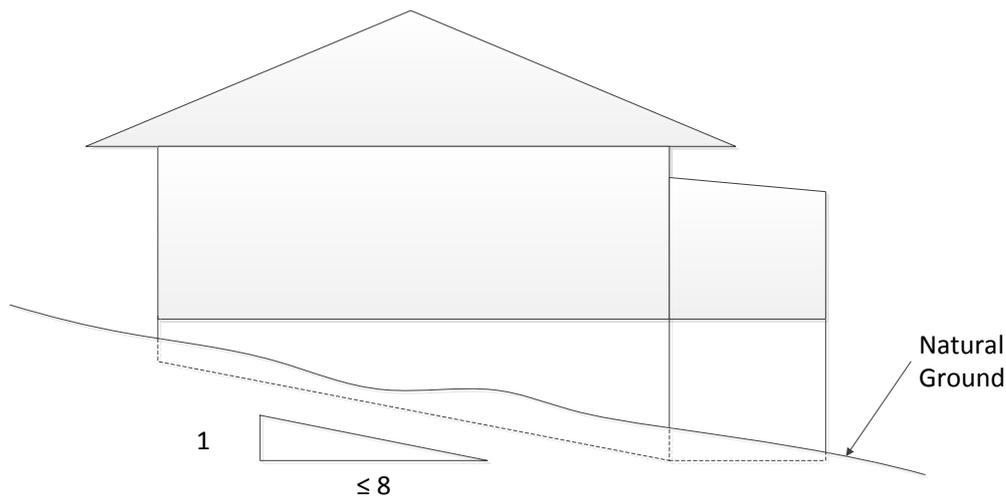
**Figure C9.2: Definition of sloping ground**
