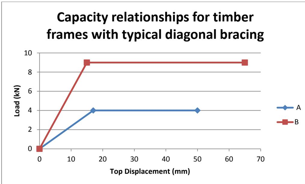
**Figure C9B.3: Capacity relationships for 2.4 m high timber frames with diagonal bracing as noted below**
