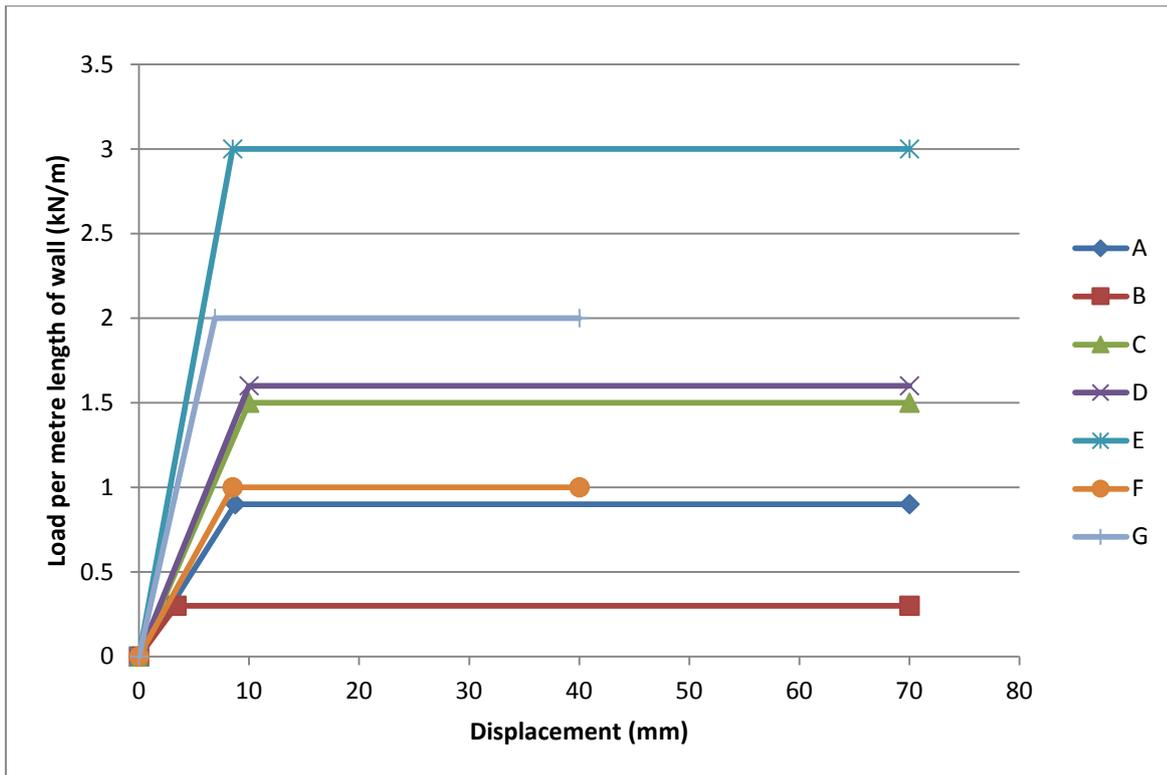
**Figure C9B.2: Capacity relationships for 2.4 m high timber framed walls with sheathing materials as noted below**
