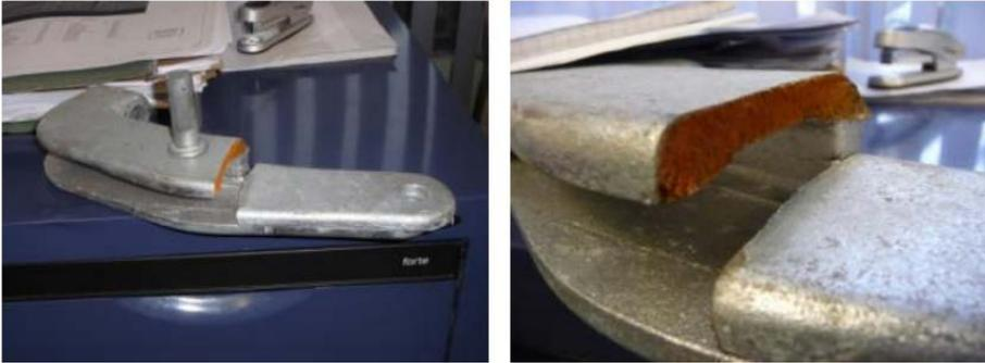
**Figure C6.6: Proprietary brace connectors that failed during the February 22, 2011 Christchurch earthquake (Clifton and El Sarraf, 2011)**
