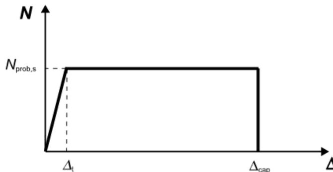
**Figure C6.11: Force-displacement relationship for steel braces in tension**
