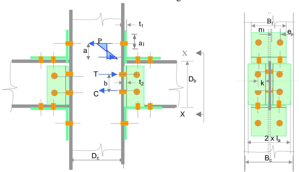
Figure C6.16: A clip angle riveted connection
