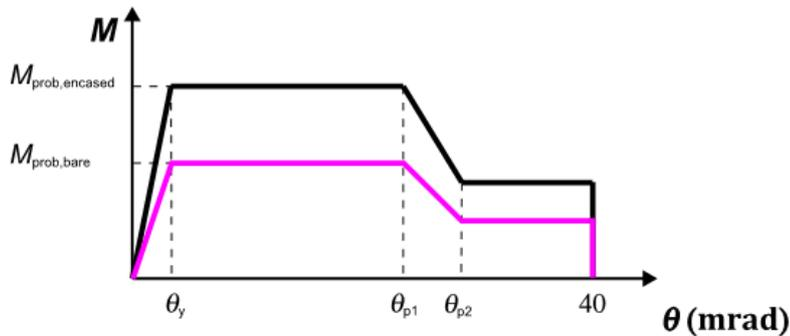
Figure C6.17: Moment-rotation behaviour of clip angle connections
