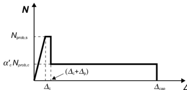
Figure C6.10: Force-displacement relationship for steel braces in compression
