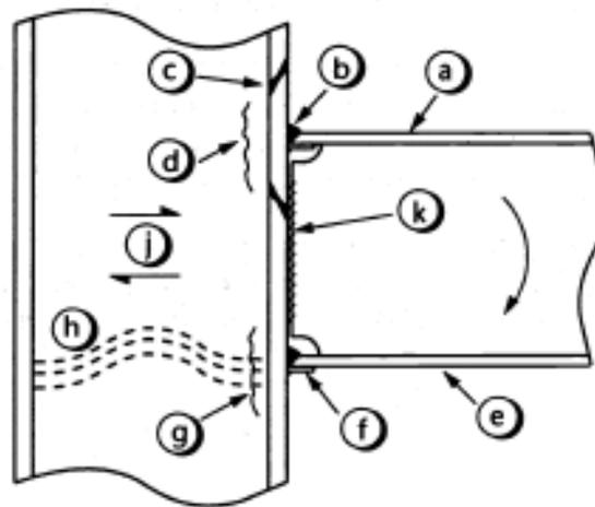
Figure C6.18: Components of welded connections requiring checks (SCI, 1995)
