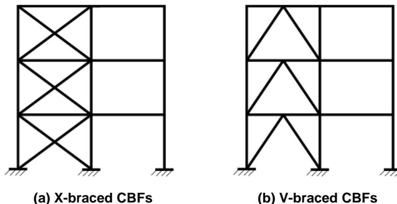
Figure C6.20: Concentrically braced frames (CBFs)
