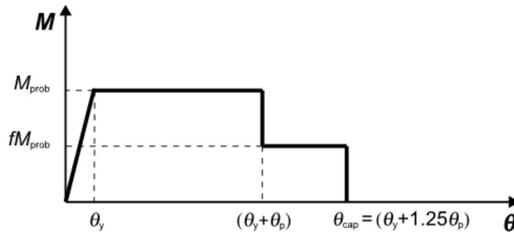
Figure C6.9: Moment-rotation relationship for steel beams and columns with FLR
