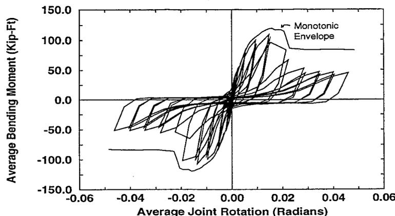
Figure C6.14: Comparison of monotonic and cyclic moment–rotation behaviour
