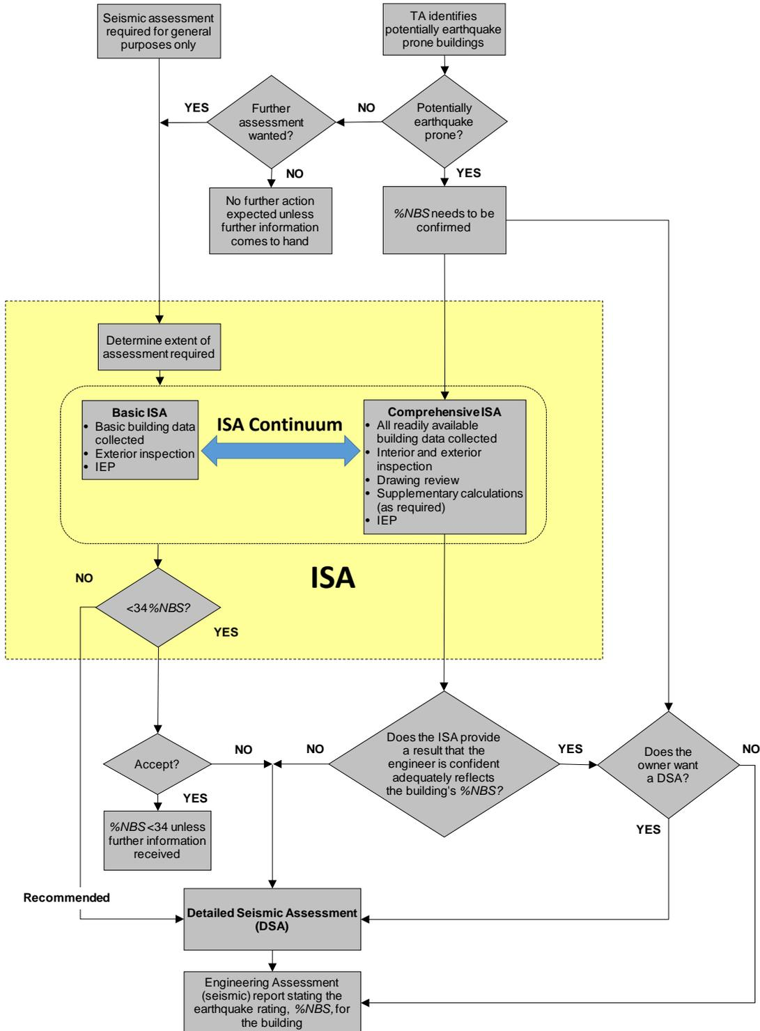
Figure B.1: Diagrammatic representation of the Initial Seismic Assessment process
