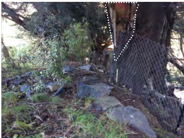
Photo B3: Tree impact damage (outlined) from boulder impact (note that the boulder has been mechanically broken up after impact).
