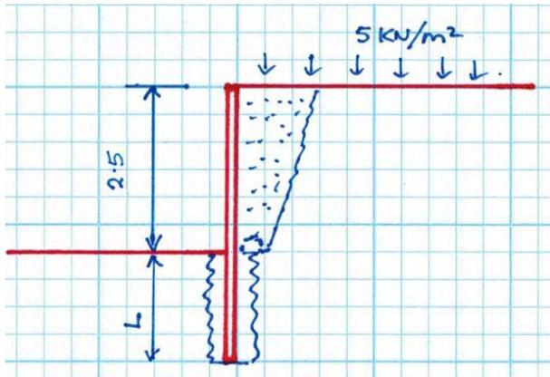
Figure B.3: Gross pressure method of analysis for embedded cantilever wall (gravity case)
