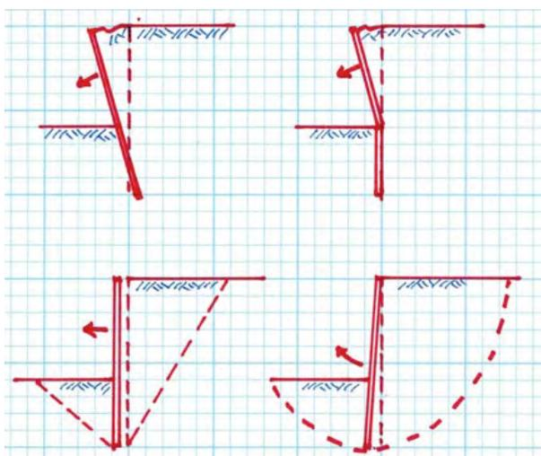
Figure B.2: Cantilever pole retaining wall example
