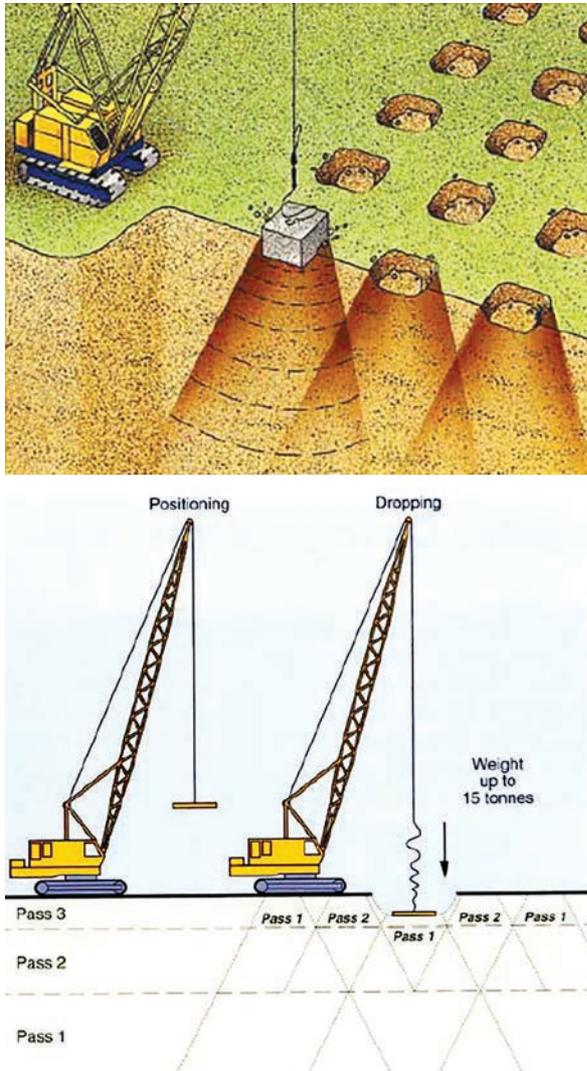
The number of passes, drops and drop spacing is calculated initially based on the estimated total energy needed to treat the soils. Grid spacings, drop heights and number of drops are then confirmed with a field trial prior to commencing production ground improvement. Initial estimates of the required energy for treatment can be taken from Figure A.4.3.
