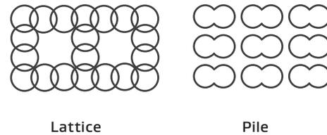
driven piles, there is added benefit of densification of soils between the columns. Jet grout columns can be reinforced by plunging a cage into the wet slurry similar to the reinforcement of CFA piles.
