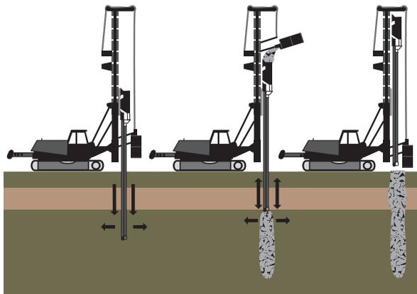
**Figure 7.11: Rammed aggregate pier construction using displacement based method (after Wissmann et al, 2015)**
