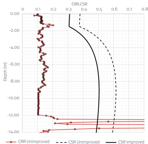
As CRR unimproved is below CSR improved, the design cannot rely solely on reinforcement affects to prevent liquefaction of the soil between the columns in a ULS earthquake. CRR of the improved ground needs to be quantified with a field trial to determine whether the design has the required factor of safety against liquefaction for soils between the columns.
