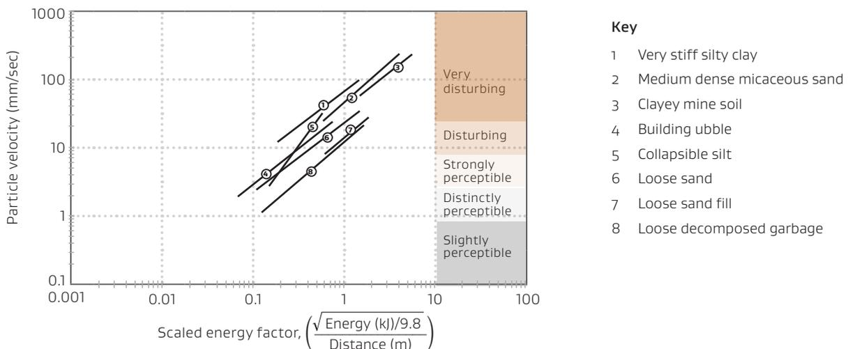
**Figure 7.2: Construction vibrations (Mosely and Kirsch 2004)**
