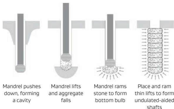
Vibrations may be a nuisance to neighbouring properties but are generally less than those from impact methods like dynamic compaction. As with vibro-compaction, turbid water from installation of the stone columns needs to be managed during construction.
