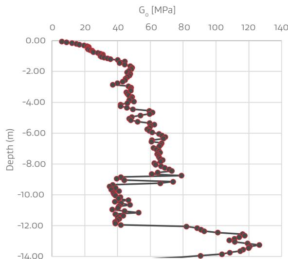
For this example,  $G_o$  is calculated using the correlations by Rix and Stokoe (1991) for soils with  $I_c < 2.6$ :
