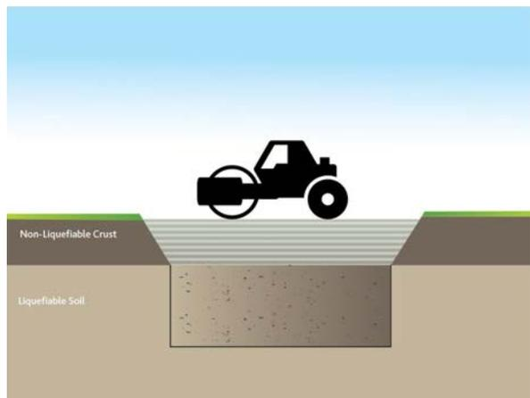
**Figure 11.2: 'Crust reinforced with inclusions' residential ground improvement options**
