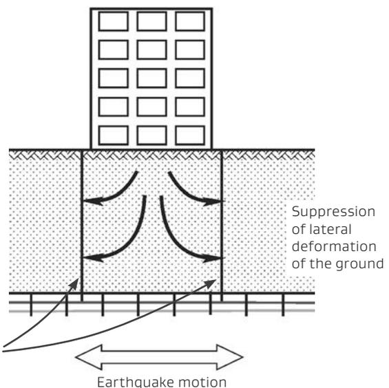
With lattice reinforcement, the lattice perimeter wall can often be placed below the perimeter of the building unlike most densification and drainage methods. This is advantageous for ground improvement beneath buildings constructed close to the legal boundary.
