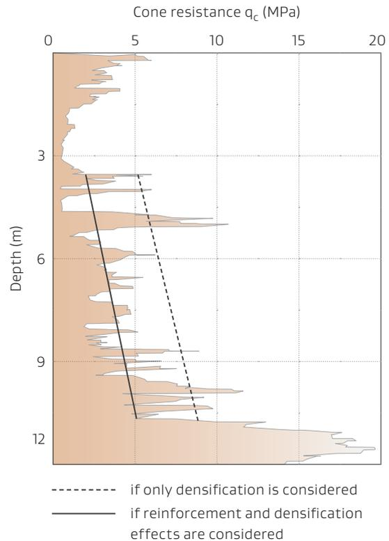
**Figure 7.4: Example of a stone column field trial**
