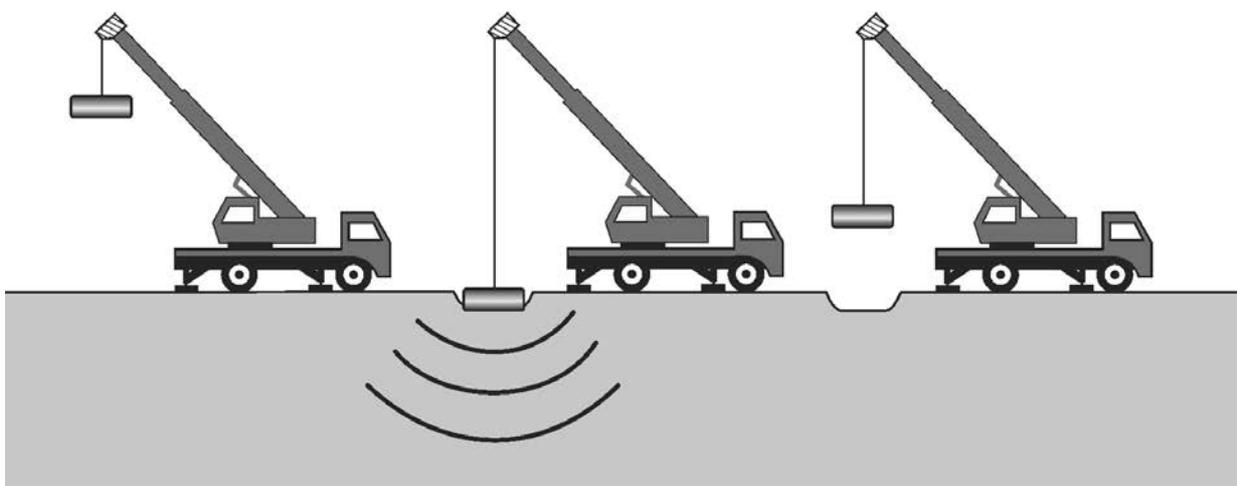
**Figure 7.6: Soils suitable for dynamic compaction**
