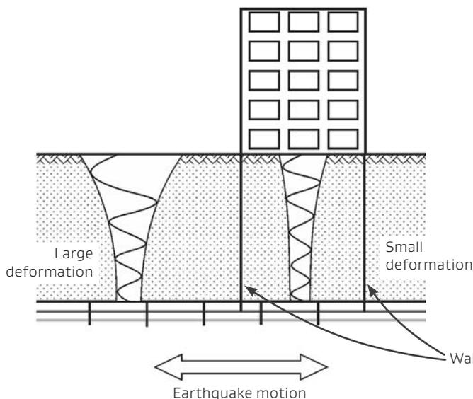
**b suppression of lateral flow of ground after liquefaction (after JGS 1998)**
