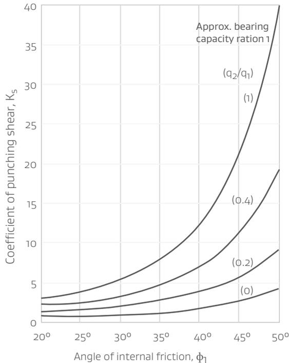
$q_1, q_2$  = ultimate bearing capacity of a strip footing of width  $B_f$  on the surface of the improved zone and on the surface of the liquefied soil respectively.
