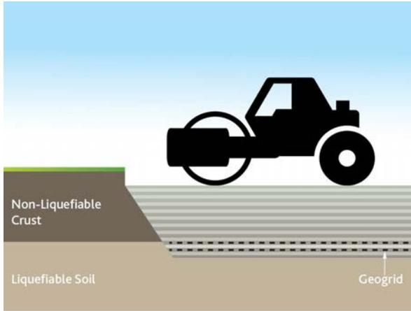
Rapid impact compaction/dynamic compaction
