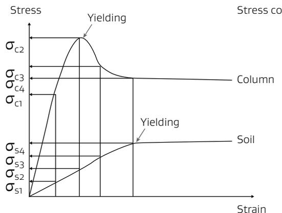
In this example, the in situ peak angle of shearing resistance is considered reasonable to assume for the surrounding soil. However, we note that there may be some improvement in strength from densification with the installation of the columns. The composite strength of the upper two layers is therefore calculated as:
