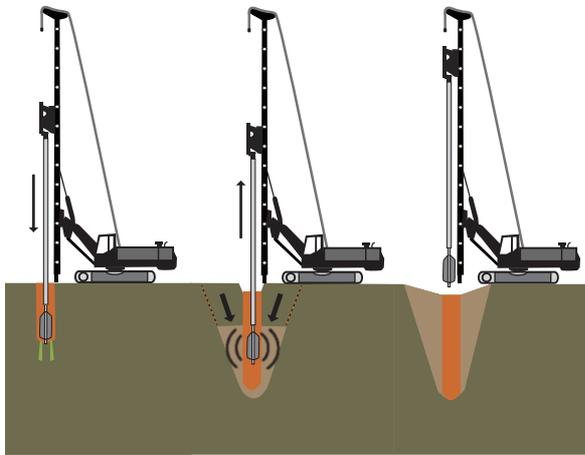
The degree of compaction generally decreases with increasing distance from the probe. Establishment of the treatment spacing, frequency of the vibrator and advancement and withdrawal rates is based on past experience or a field pilot study. Spacing of the treatment grid can initially be estimated from Figure 7.9. Other useful charts for determining a treatment spacing are in JGS 1998.
