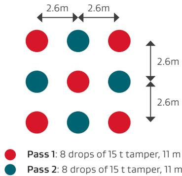
For eight drops of a 15 t hammer from a height of 11 m, the estimated crater depth is therefore:
