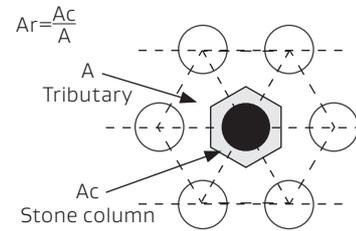
A symmetrical pattern is selected for the stone column arrangement so that stiffness is uniform. Columns are typically installed in a square or triangular grid as shown in Table A.3.2.
