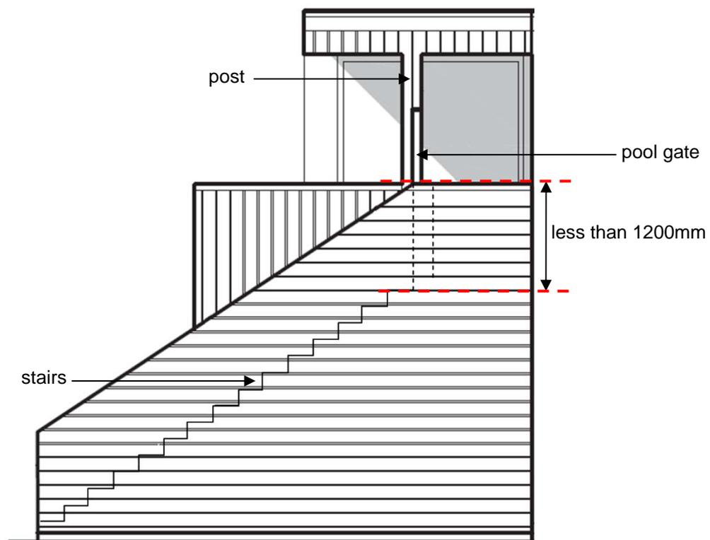
**Figure 2: Elevation showing gate and stairs (not to scale)**
