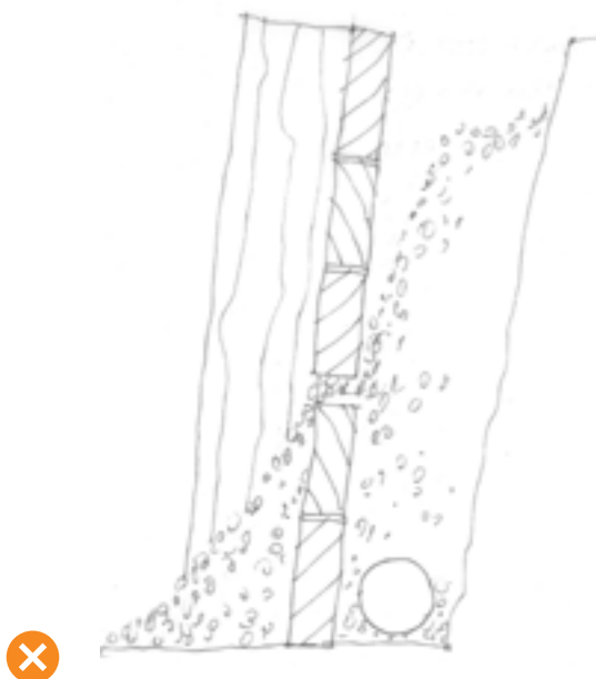
Figure 4 Coarse fill passing through a timber retaining wall.
