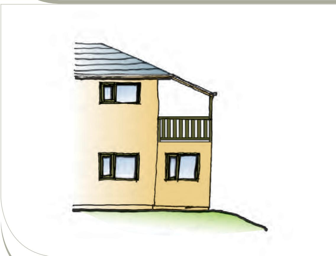
Figure 7.4 Solid balustrade replaced to allow at least one side of the deck to be open.
