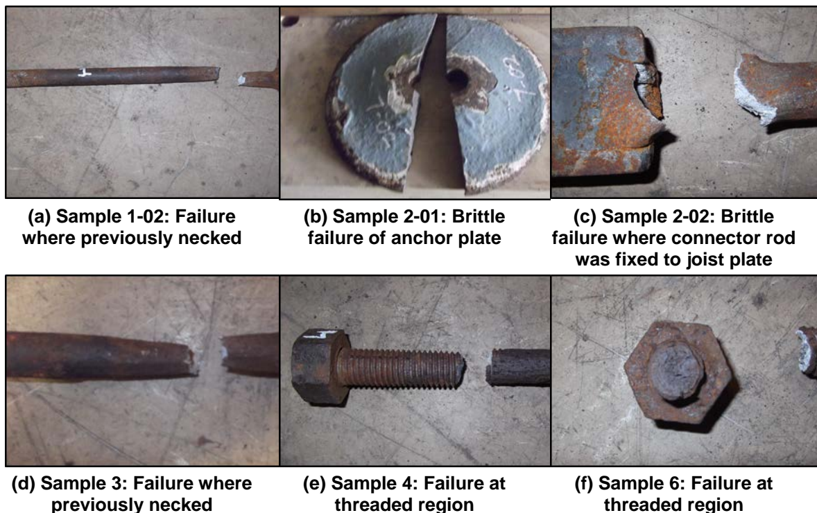
Figure C8.36: Observed failure modes from tensile test series (Campbell et al., 2012)
