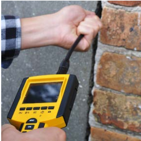
(a) Borescope inspection camera
