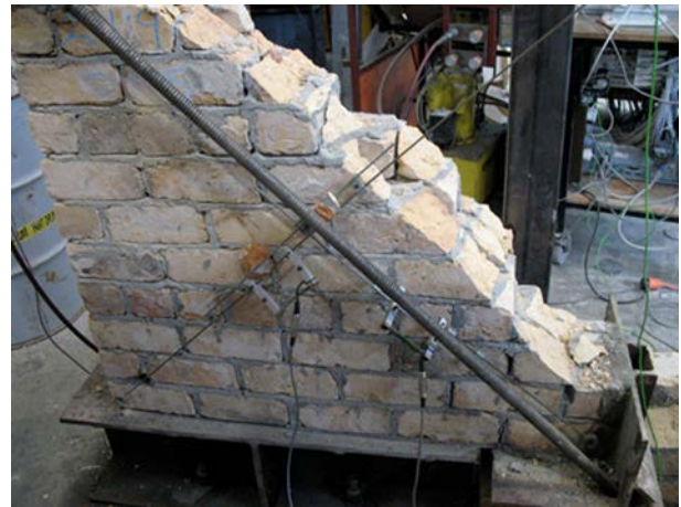
(a) Diagonal tension cracks to a brick pier. Note splitting of bricks (Dizhur)
