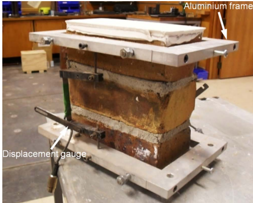
Figure C8A.1: Example of extracted sample with test rig attached for the prism compression test
