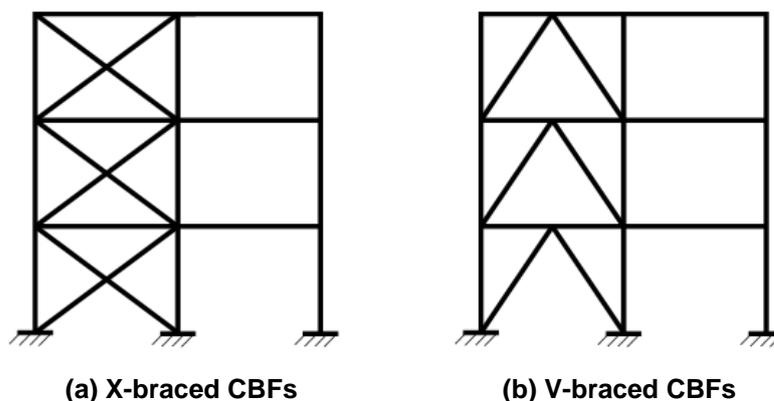
Figure C6.20: Concentrically braced frames (CBFs)
