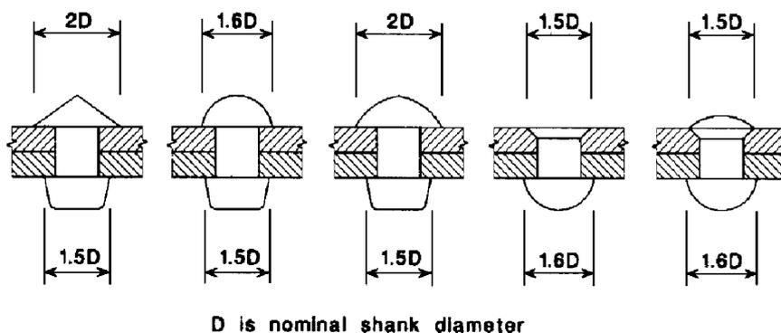
Figure C6.13: Typical rivet shank and head diameters (Bussell, 1997)
