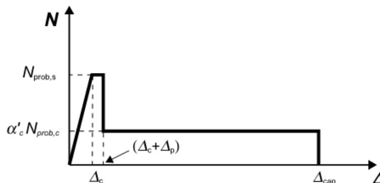
Figure C6.10: Force-displacement relationship for steel braces in compression
