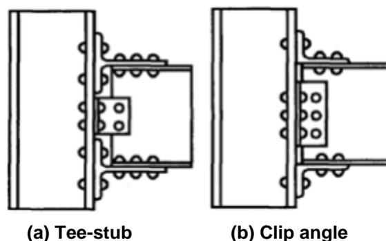
**Figure C6.12: Typical riveted connections (Roeder et al., 1996)**
