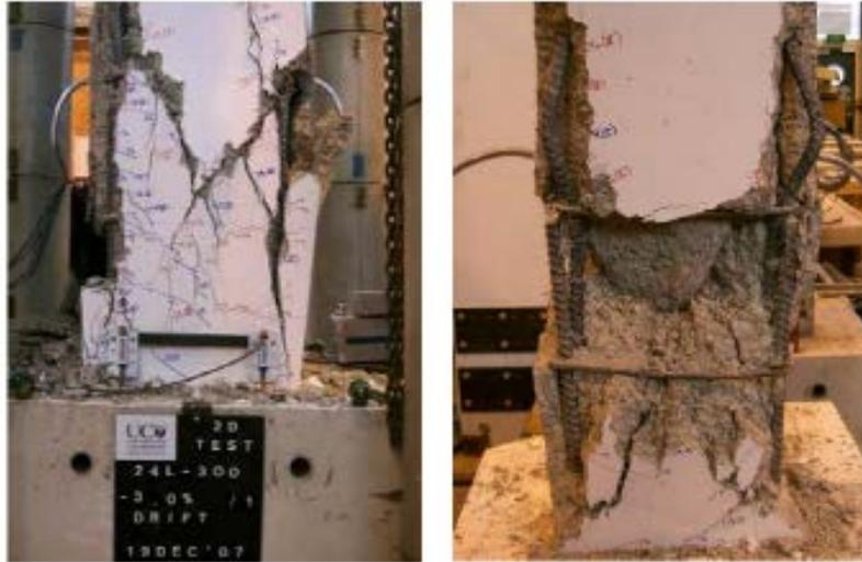
**Figure C5.2: Performance of poorly detailed and confined gravity columns designed according to NZS 3101:1982 code provisions (after Boys et al., 2008)**
