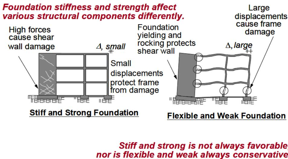
**Figure C4.4: Influence of SSI on structural performance (figure adapted from Mahoney, 2005)**
