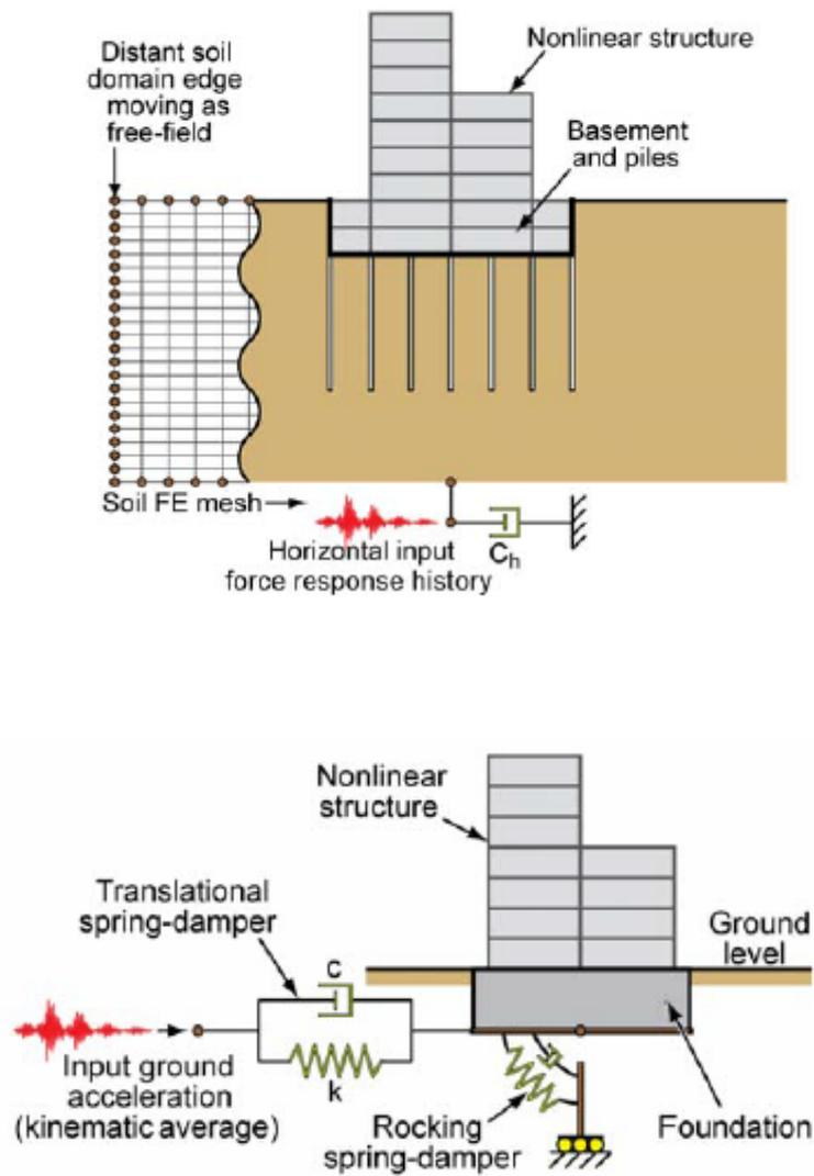
Figure C4.6: Direct and indirect SSI modelling (Deierlein et al., 2010)
