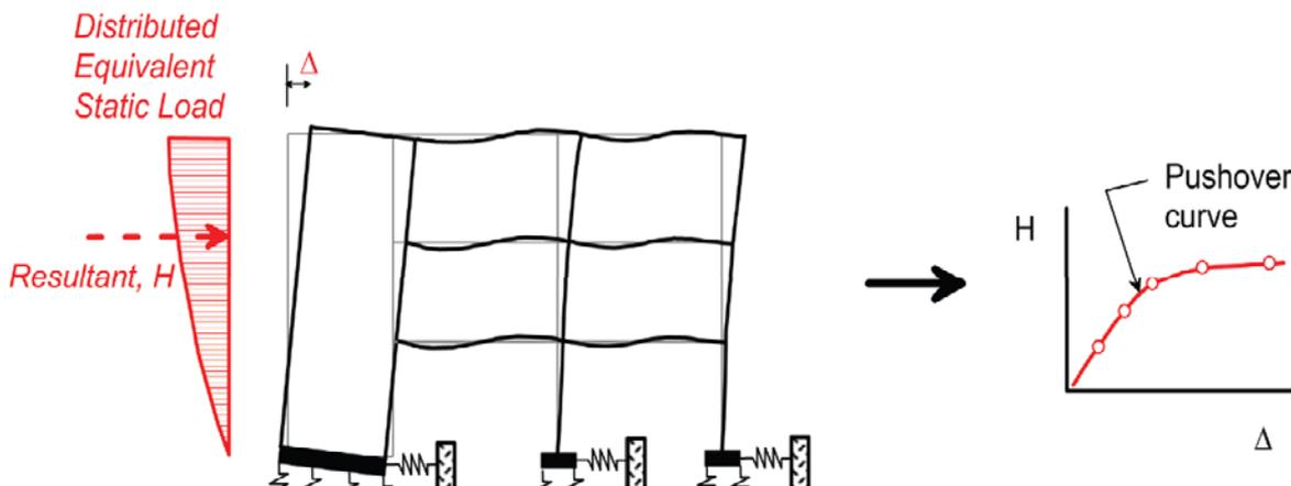
Figure C4A.2: Schematic illustration of a pushover analysis and development of a pushover curve for a structure with a flexible base (NIST, 2012a)
