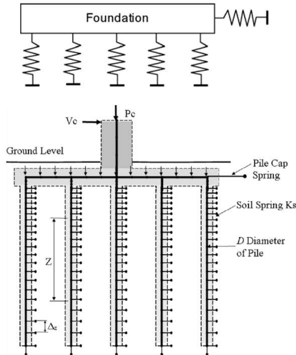
**Figure C4A.1: SSI model for flexible base model using Winkler spring for shallow foundation and deep pile foundation**
