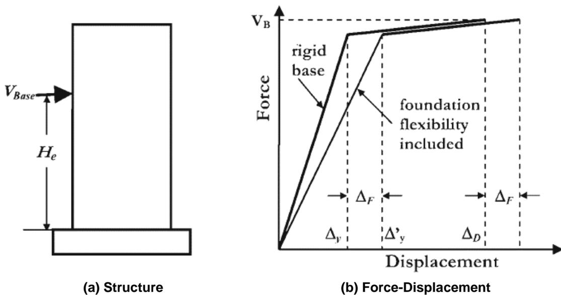
**Figure C4.5: Influence of foundation flexibility on displacement and ductility capacity in the structure**
