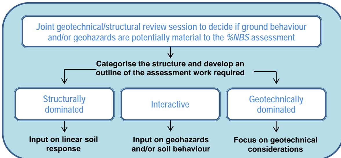
**Figure C4.1: Project categorisation to reflect potential impact on the assessment of geotechnical issues**
